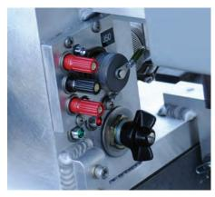
Seven isolated firing circuits are distributed on the F6+ arm and rear, allowing convenient and easy access.
